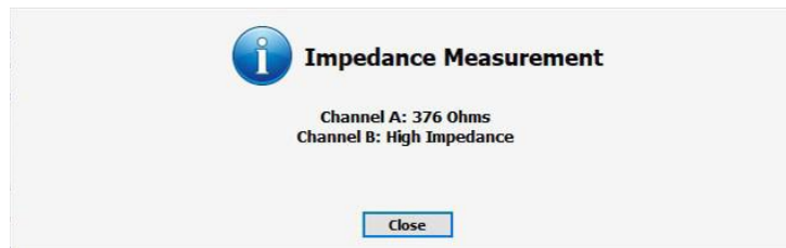
Figure 11: Impedance Measurement pop-up Window, Channel A only
